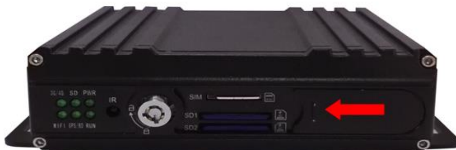
Figure 6. SD card installation
