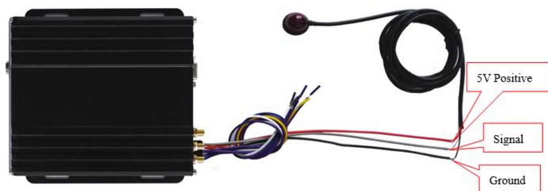
Figure 12. IR extension connection
