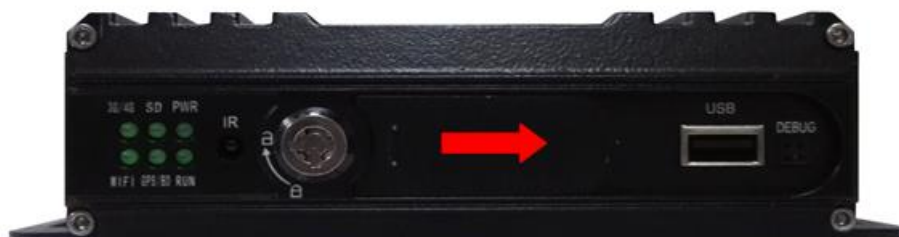
Figure 5. SD card Installation
