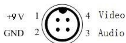
AV-OUT Monitor Interface
